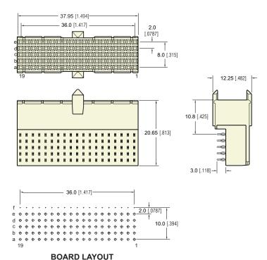
The **E-Z met** Type AB-19 connector provides 95 contacts as well as pre-alignment guides. These connectors are available either with or without integrated upper ground return shields. Lower ground return shields may be ordered separately.
