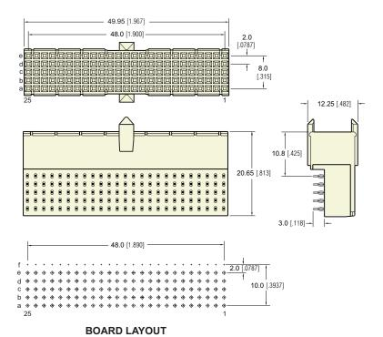
The **€-Z met** Type AB-25 connector provides 125 contacts as well as integrated pre-alignment guides. These connectors are available either with or without integrated upper ground return shields. Lower ground return shields may be ordered separately.
